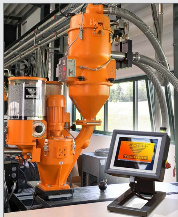
G-mixer with two Kö dosing stations and the new SLT and MCT control units with 7," colour touch display
